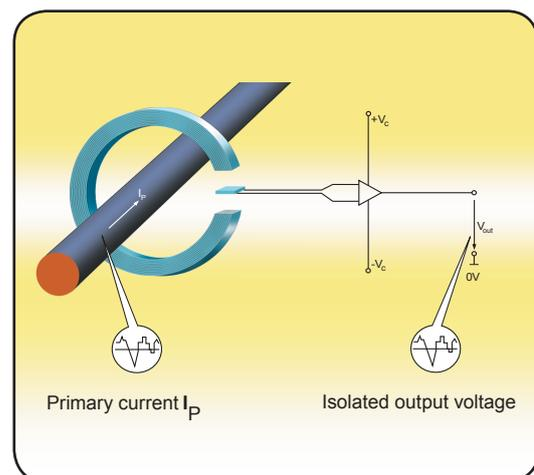
Fig. 1: Principle of the open loop transducer
